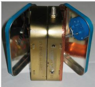
A view of both tins open. Notice the copper tape shielding on the right-hand tin.
