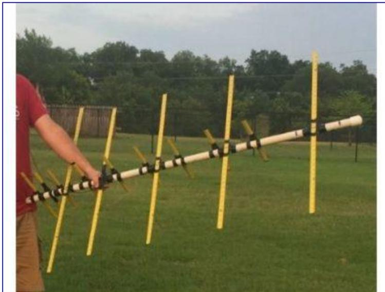
The element holders are attached to the boom with electrical tape in the photo above. While I haven't tried it, I'd suggest that the antenna might be a bit more robust if you could screw or perhaps glue the holders to the boom.
